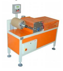
The automatic machine mod. SGT 40 cuts the paper and fibre wound on a 500mm diameter reel. It is able to cut pieces up to a maximum length of 850 mm and to create compact stacks of the cut product. Up to 20 sizes can be saved, which can be edited at any time; other sizes can be created on a case-to-case basis as an alternative to the twenty stored. The SGT 40 paper cutting machine can also be programmed to cut in order for different quantities and sizes.
