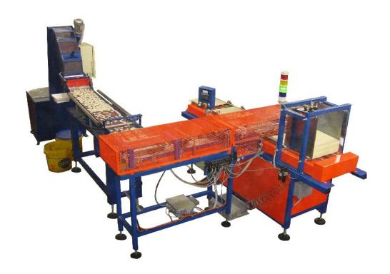
Loading machine mod. SGC automatically loads mosaic inserts (square shaped) in templates with the help of just one operator who sorts the piece before it is placed in the mold, in order to speed up the work of the operator in charge of final product inspection and to increase production by eliminating pieces that could cause the machine to stop.
